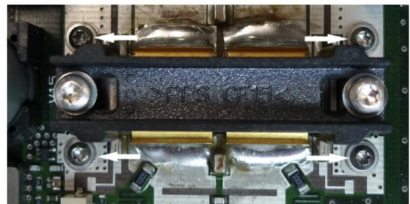
Figure 4-51: Tightening screws of ground strips
