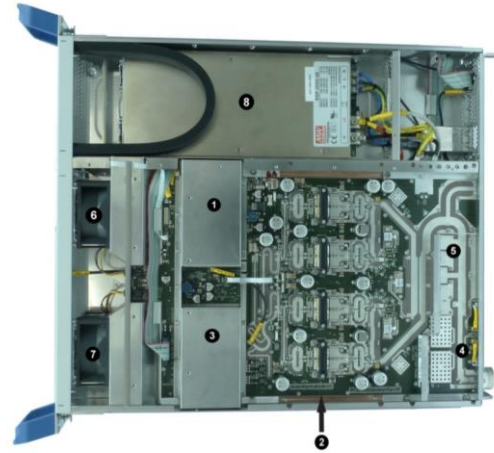
Figure 3-3: Amplifier board - A2 (top cover removed)
