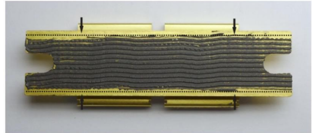
Figure 4-47: Spreading heat-conducting paste
